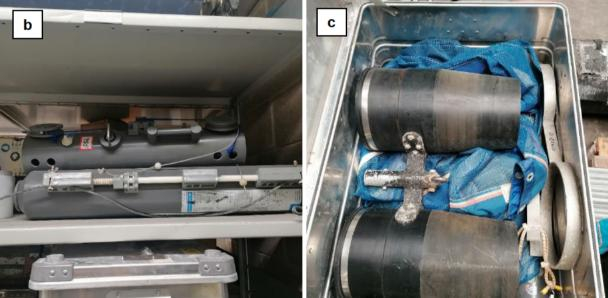
Figure 1: panel a (top) – frame for optical profiler, b (bottom left) – GoFlo bottles, c (bottom right) – miniBongo net with 100 um mesh net.
